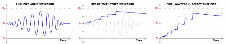
This voltage range is then sent to a difference amplifier (OPA277 single op-amp) that subtracts about 6 volts from it, and amplifies the result by a 1.75 voltage gain. The subtracted voltage reference is programmed by a 10k pot, allowing one to account for the minimum engine noise level.
