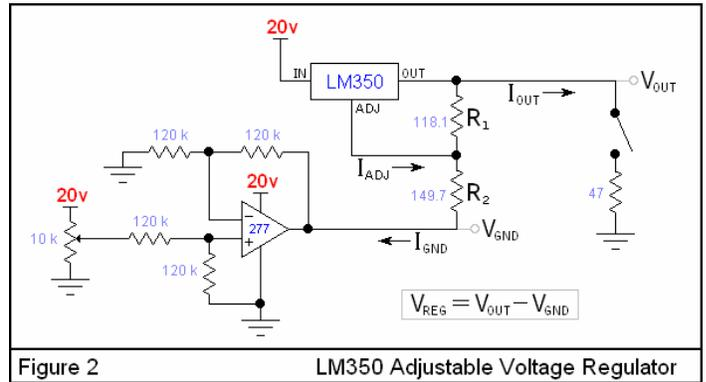
Figure 2 LM350 Adjustable Voltage Regulator
